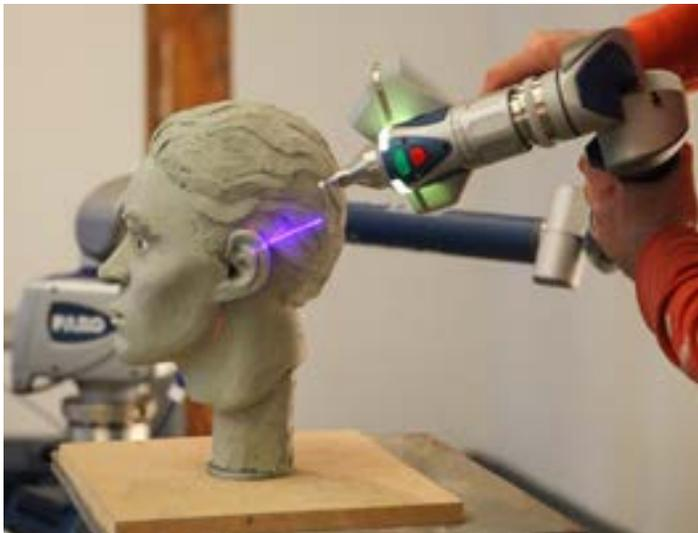
The non-contact laser measurement process used by the FARO ScanArm makes it ideal for preserving a digital model of skulls. It took approximately five minutes to fully document each bust with the FARO ScanArm.
