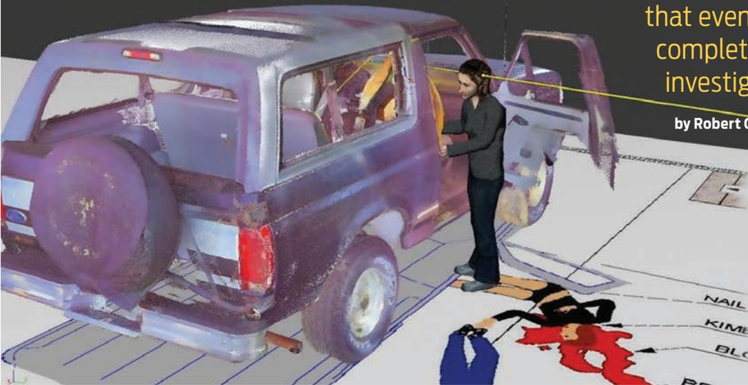
■ The crime scene recreation image shows 3ds Max software with the point cloud being created with a FARO Laser Scanner and processed in FARO SCENE software.
