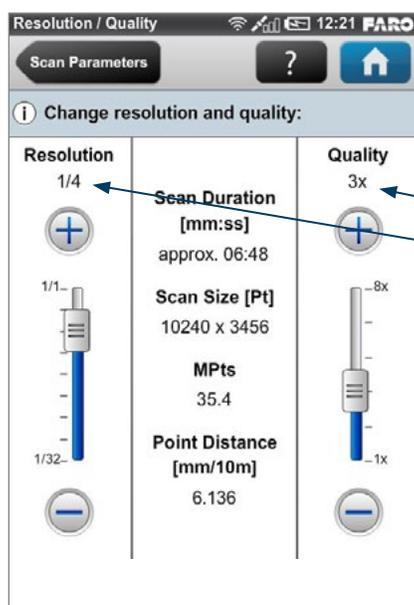
Figure 11. FARO scanner Resolution / Quality setting screen.
