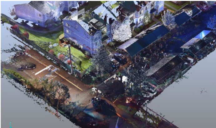
Figure 5. This point cloud was created from 35 scans at a large, multiple homicide crime scene. It was the first time the Federal Way Police Department's FARO Focus3D S 120 Laser scanner was used as part of an investigation.
